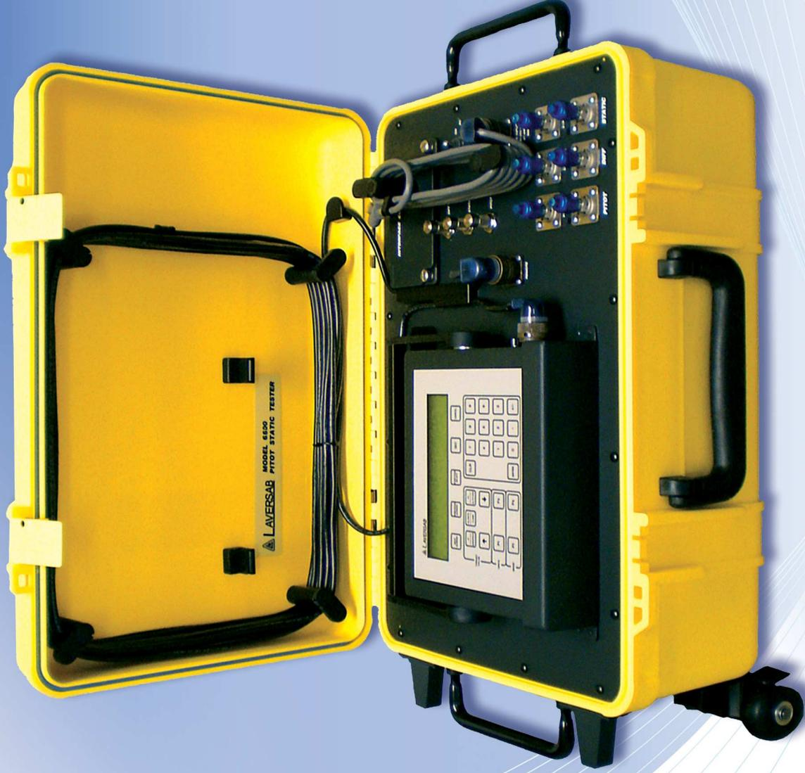
**Pitot Static Tester: 3-Outputs**
